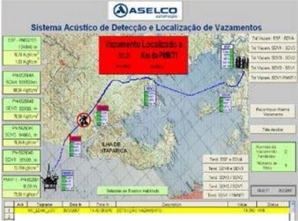
System configuration and operation are performed on a dedicated computer running non-proprietary supervisory software. It acts as a Human-Machine Interface (HMI) and features customized pictographic screens illustrating pipeline aerial views and highlighting the monitored points and many other vital system details.
